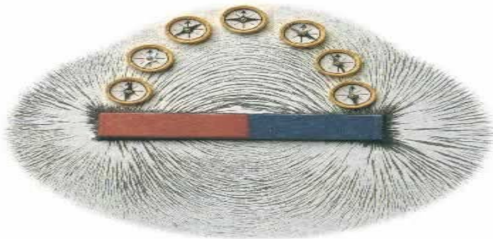
Iron filings and compasses show the shape and direction of the magnetic field
